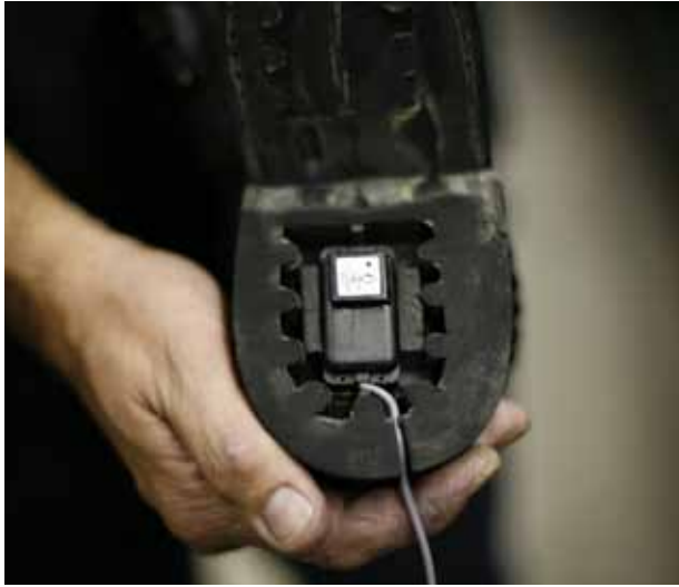
IMU and miniaturized radar sensors are embedded in a boot.
