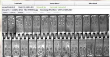
Belt Inspection system reveals flaws before expensive breakdowns
