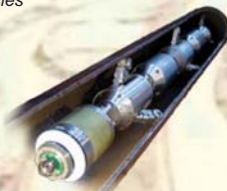
The Explorer robot travels untethered through pipe networks to inspect for problems
