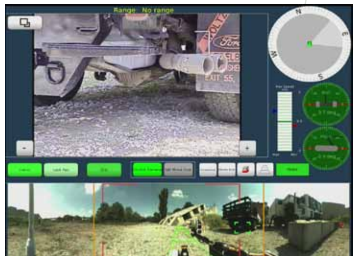
Operators can zoom in on areas like the underside of the truck (indicated by the green brackets on the bottom right). The camera automatically adjusts its contrast for darker areas.
