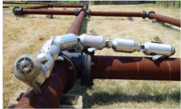
Figure 3 : Explorer - Pipe Inspection System
