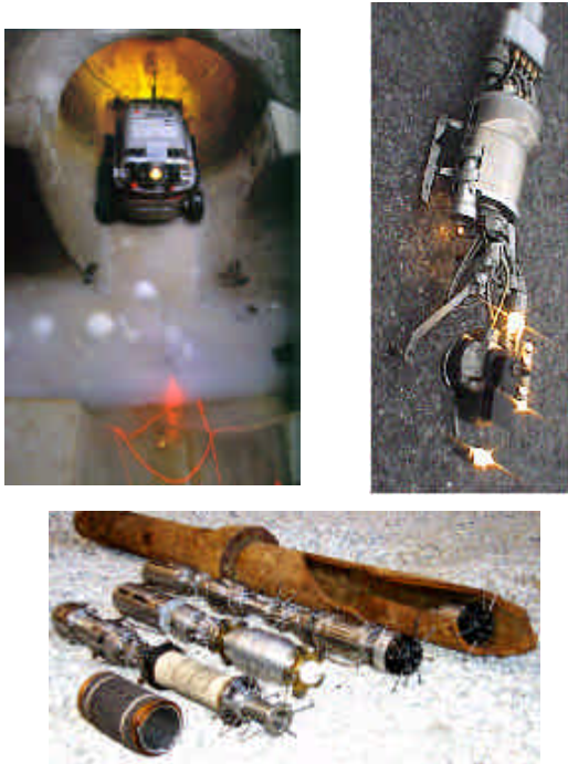
Figure 2 : Tethered gasmain ( CISBOT - right; GRISLEE - bottom) and untethered autonomous ( Kurt I ) robots developed to date by industry and researchers
