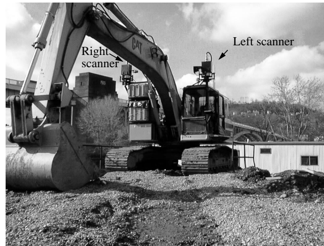
Figure 2. Sensors mounted on excavator.
